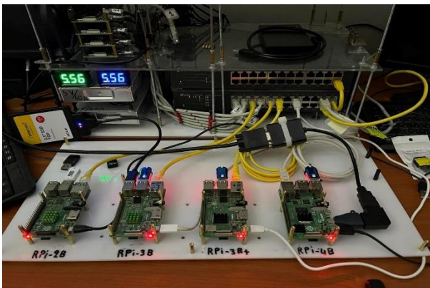
Figure 6: Single Board Computers (SBC) – RPi 2B vs RPi 3B vs RPi 3B+ vs RPi 4B.
