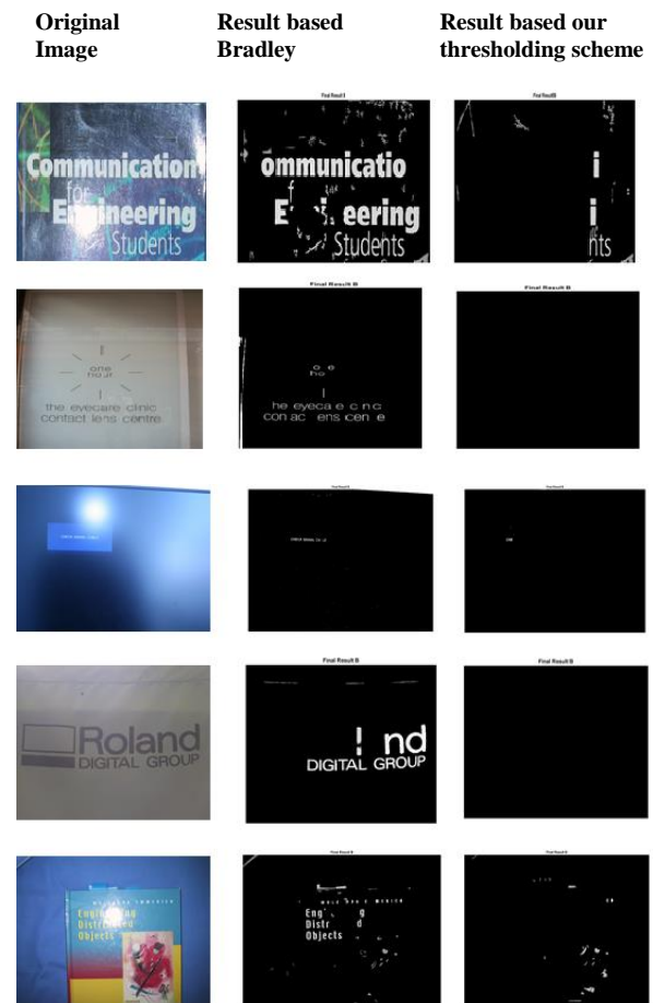
Fig 5: Samples images show that the using of adaptive thresholding is better than our thresholding method
