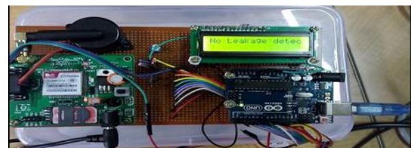
Fig. 6. The Arduino UNO and LCD screen connected together using a prototyping breadboard
