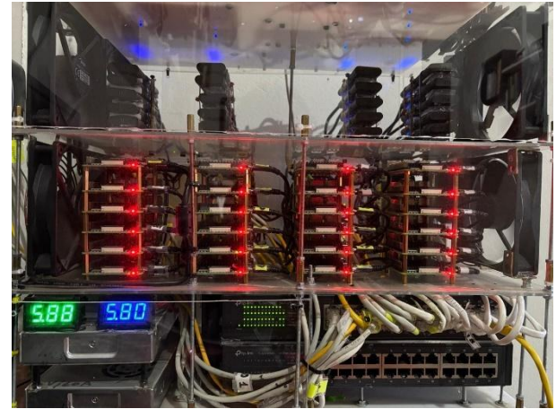
Figure 2: Deployment of the Beowulf Cluster with (24) RPi-4B (8GB)
