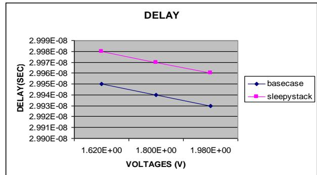
Fig 11: Impact of voltage on write delay
