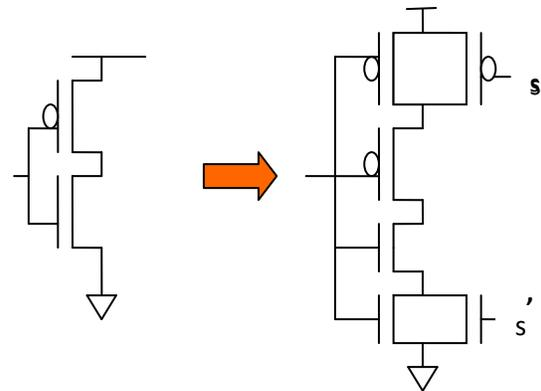
Conventional CMOS Inverter      Sleepy Stack Inverter
