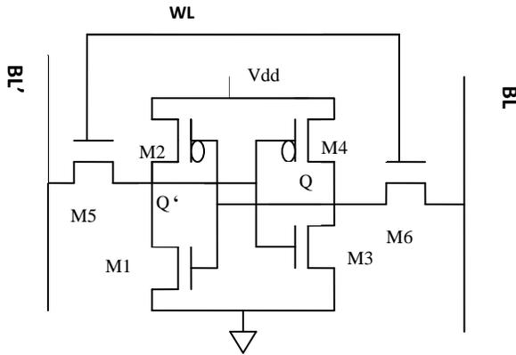
Fig 4: Conventional SRAM Cell
