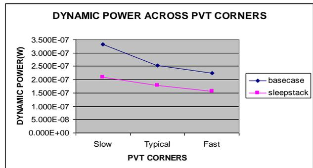
**Fig 7: Dynamic power comparison graph across PVT corners for SRAM**
