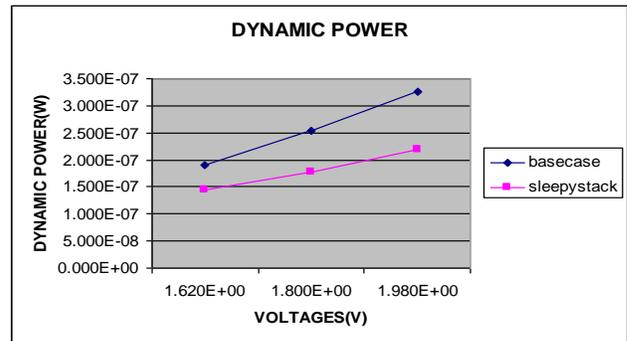
Fig 10: Impact of voltage on dynamic power
