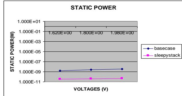
Fig 9: Impact of voltage on static power
