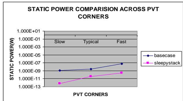
**Fig 6: Static power comparison graph across PVT corners for SRAM**
