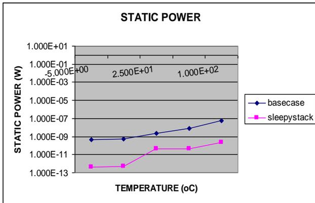
**Fig 12: Impact of operating temperature on static power**
