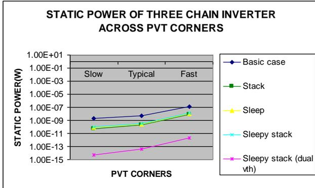
**Fig 1: Static power comparison graph for various design cases across PVT condition for three chain inverter**
