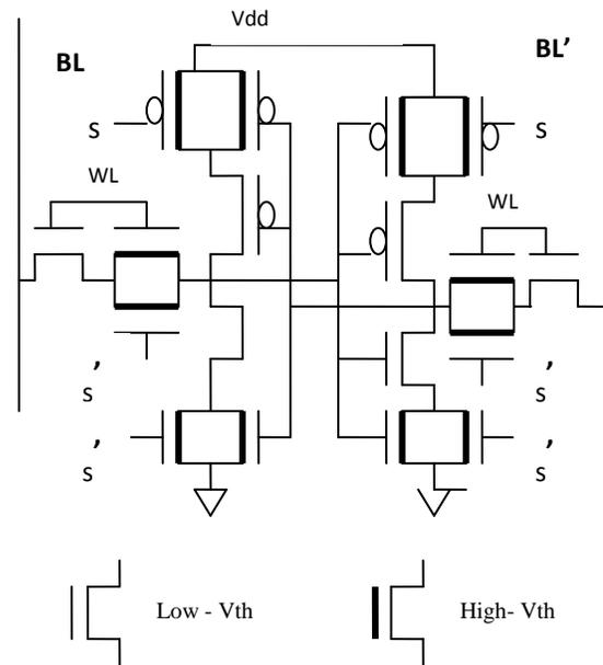
Fig 5: Sleepy stack SRAM cell
