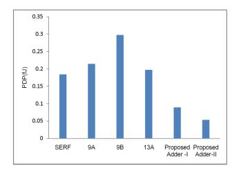
Fig 4: Comparison of PDP of Different Full Adders
