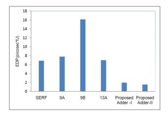
Fig 5: Comparison of EDP of Different Full Adders
