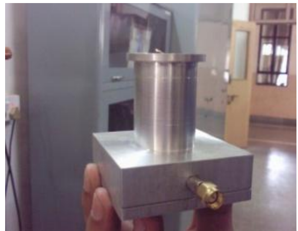
Figure 6 helical loaded cavity backed antenna, 60 mm rectangular base
