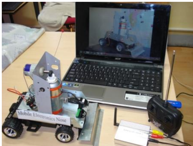
Figure 7. Image of developed mobile Electronic-Nose with computer and remote control setup in NEHU Shillong, India.
