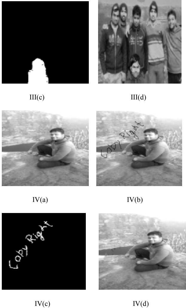
Fig 4: Embedding, Alteration, Detection and recovery of watermarked image.
