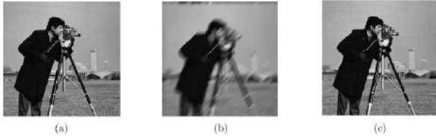
Fig 2: Results obtained using direct inverse filtering (a) Original image, (b) Blurred image, (c) Inverse filtered image.
