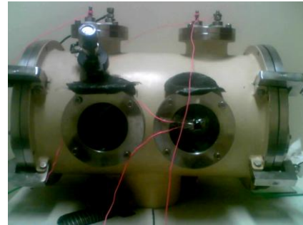
Figure 1. The experimental setup for plasma production
