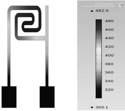
Figure 7. Simulation result(Temperature [K]) for fig(D)
