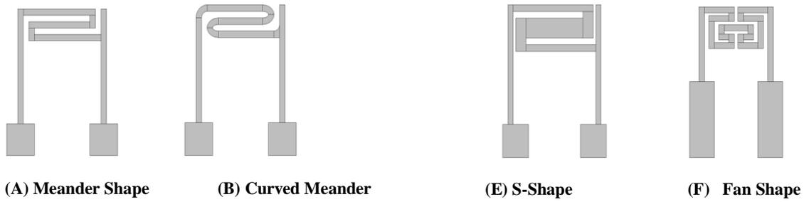
Figure 3. Six different shapes of microheater
