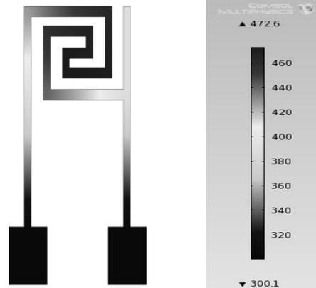
Figure 6. Simulation result(Temperature [K]) for fig(C)
