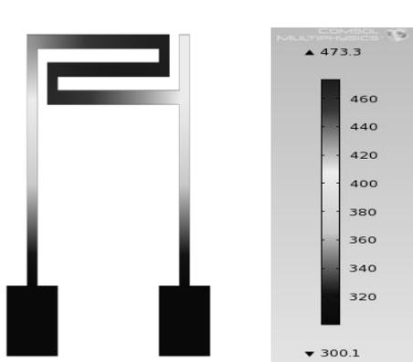
Figure 4. Simulation result(Temperature [K]) for fig(A)
