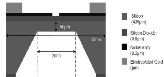
**Figure 2. Detail dimensions of the structure (Cross-section view)**
