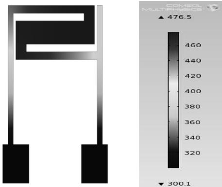
Figure 8. Simulation result(Temperature [K]) for fig(F)
