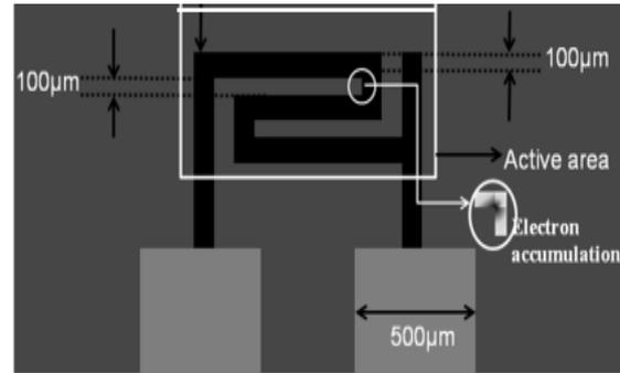
**Figure 1. Detail dimensions of the structure(top view)**
