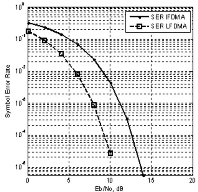
**Figure 2: Symbol error probability curve for SC-FDMA symbols using actual channel coefficients and FDE**
