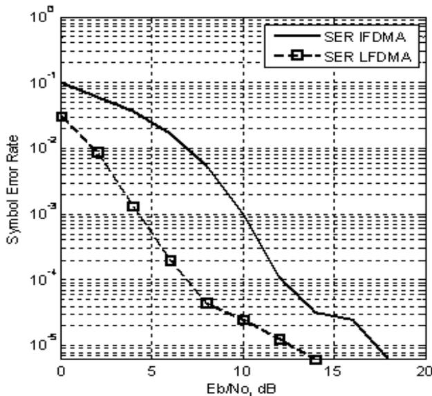
**Figure 4: Symbol error probability curve for SC-FDMA symbols using LMS channel estimation and TDE.**
