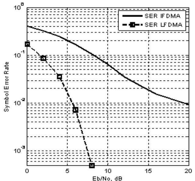
**Figure 3: Symbol error probability curve for SC-FDMA symbols using LMS channel estimation and FDE**
