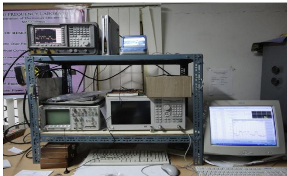
Figure 3: The experimental setup used to measure attenuation
