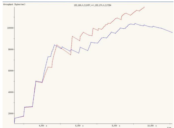
Figure 8 Throughput vs. Time Plots (First 1 M bytes in 20 MB File Transfer)
