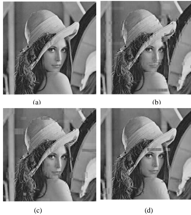
Figure 8. Reconstructed image Quality layer method (a) Original Lena, (b) without spatial Multiplexing, (c) with spatial Multiplexing, (d) with UPA
