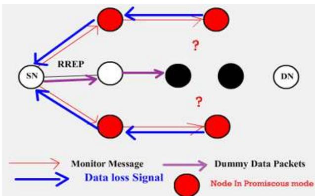
Figure 8. Propagation of Data loss Signal back to the Source Node
