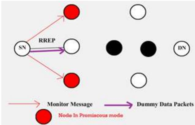
Figure 6. Propagation of Monitor message & dummy data packets
