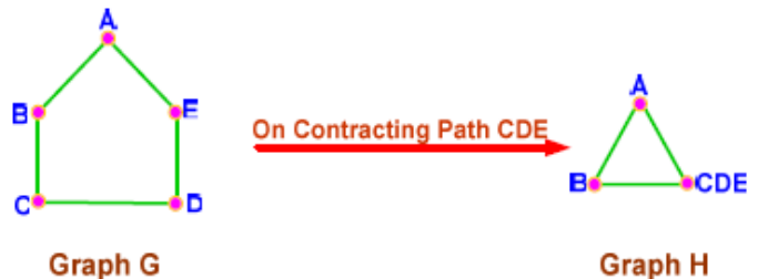
Figure 6 : Example of contracting path CDE and graph G to H
