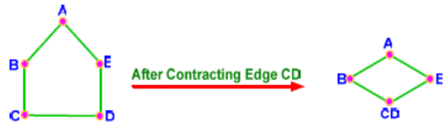
Figure 5 : Example of contracting edge CD
