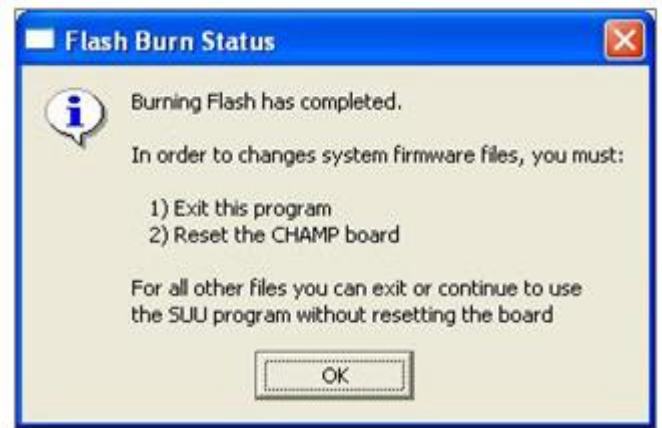
Figure 9 the output displayed on VxWorks After burning the image on ChampAV IV
