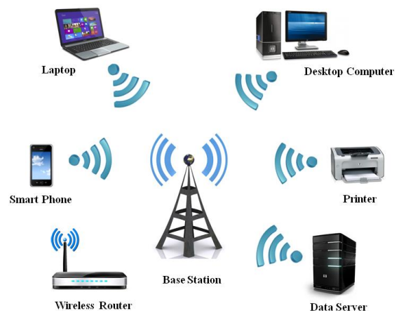
Fig.1: Typical structure of wireless network.
