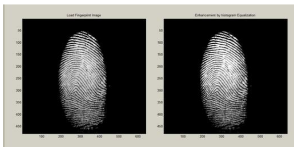
Fig 5. Image enhancement by histogram equalization
