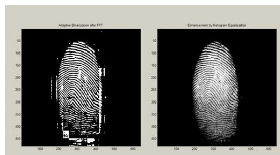
Fig 7. Fingerprint image after adaptive binarization Binarized image(left), Enhanced gray image(right)
