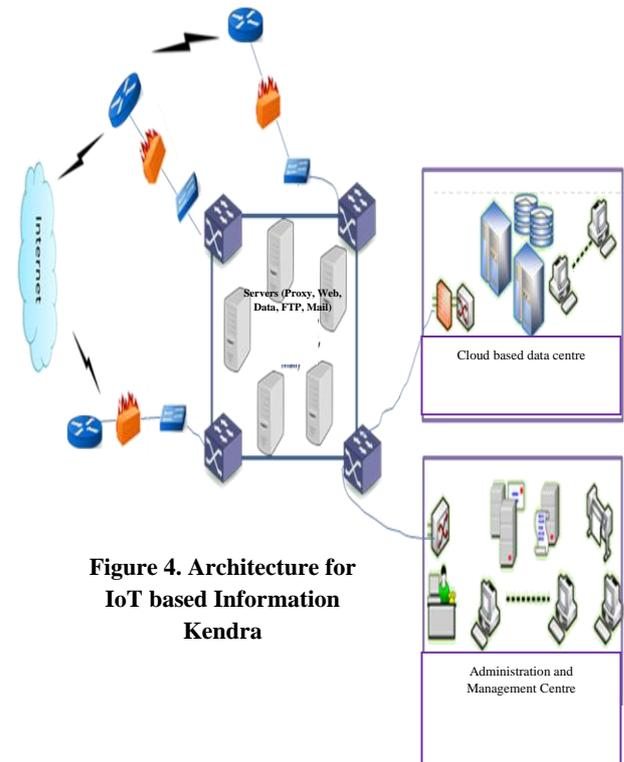
Figure 4. Architecture for IoT based Information Kendra
