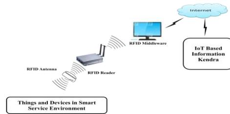
**Figure 3. RFID System**
