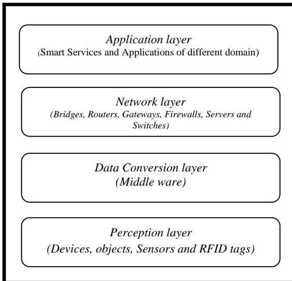
**Figure 2: Layered Framework for IoT based**
