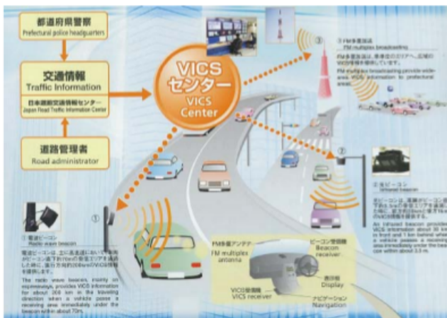
Fig. 1. Japan’s Vehicle Information Communications System (VICS)
