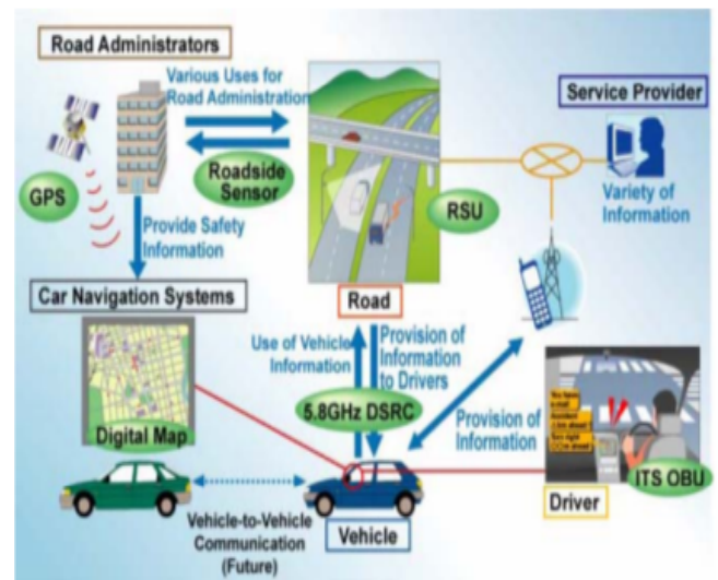
Fig. 2. Overall architecture of Smartway in Japan
