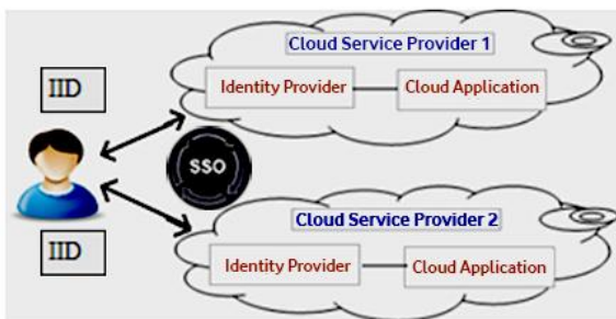
Figure 2: Architecture for inter-cloud SSO [2].
