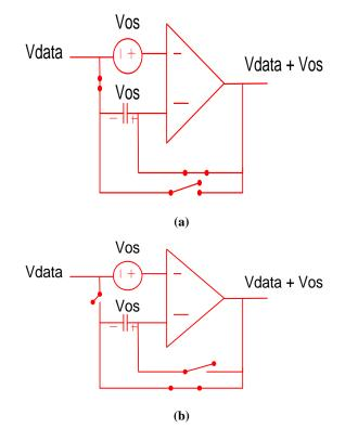
Fig. 6.Positive feedback auto zero offset cancellation structure (a) sample phase (b) output
