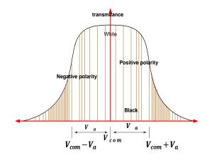
Fig 5. Luminance vs applied voltage
