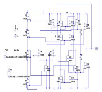
Fig 7. Schematic of proposed buffer
