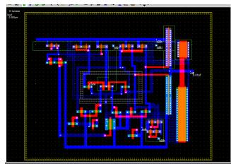
Fig 11. Layout of proposed Buffer amplifier
