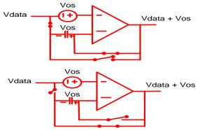
Fig 2. Auto-zero structure (a) sample state (b) output state
