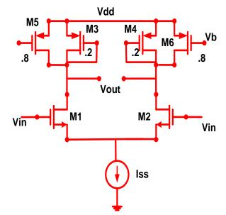
Fig 4. Differential amplifier design using current distributed load to increase the gain
