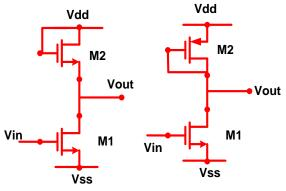
Fig 3 CS stage with diode connected load, NMOS & PMOS
