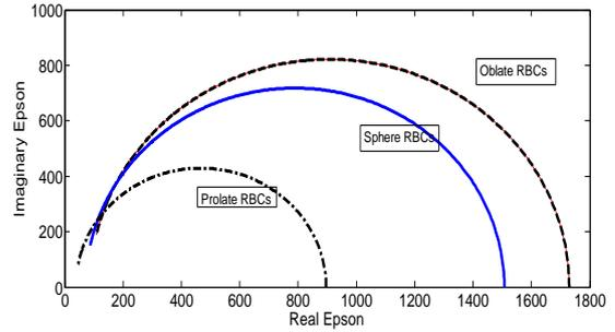
Fig.5 The dielectric response at 35% as volume fraction
