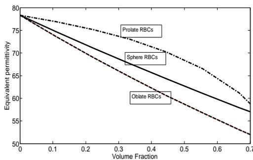
**Fig.1. The equivalent permittivity of the oblate and prolate cells with the same volume as compared to the spherical cells at different volume fractions.**
