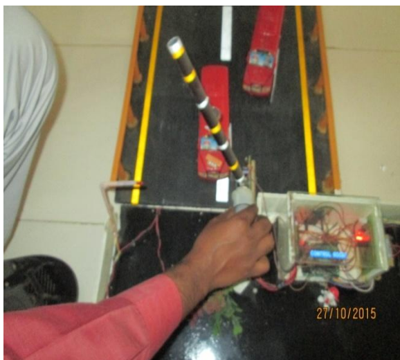
Fig.8 Bus detected , gate open state
