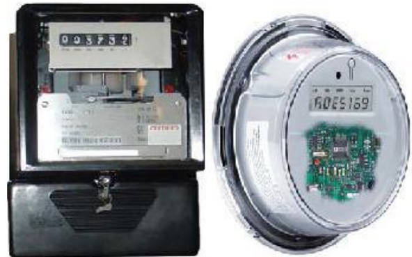
Figure 1 : Electromechanical v/s smart meter
