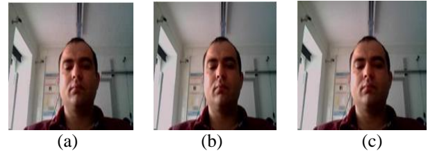
Figure 6: Comparison of Example Based Super Resolution and Reconstruction Based Super Resolution in the presence of no motion in consecutive frames. (a) Original image (b) Result of an Example-based Super-Resolution with SSIM index of 0.99. (c) Result of Robust Super-Resolution (RSR) with SSIM index of 0.98.
