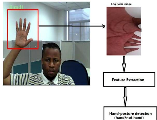
**Figure 4. The flow of hand posture detection method**
