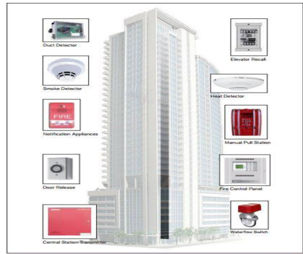
Figure 2: A typical Fire Alarm System (Source: [1]).
