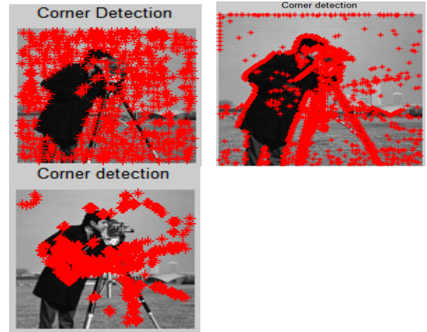
Fig 1: Comparison result of Harris (upper left), SIFT (upper right), and FAST (lower)
