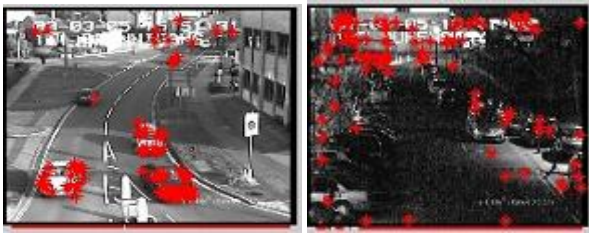
Fig 12: Corner detection of Easy, Hard, Medium and Night sequences using FAST detector
