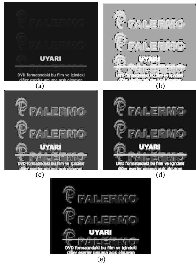
Fig.1. Results for image Palermo. (a) Original image (b) enhanced image using HE, (c) enhanced image using WTHe.(d) enhanced image using LCHM and (e) enhanced image using HEFGLG
