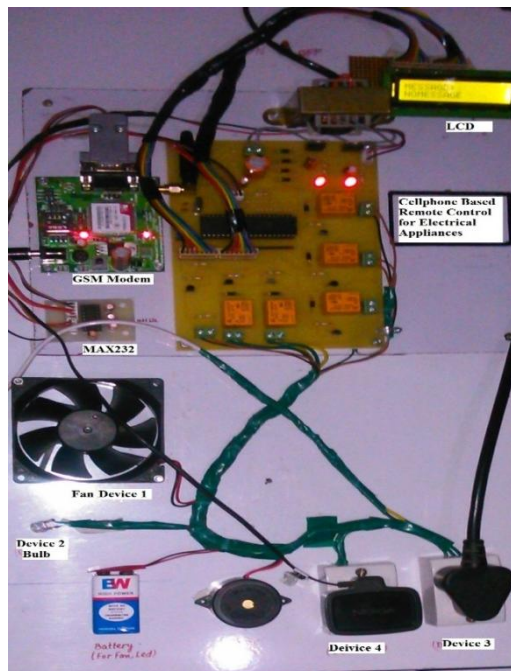
Figure 6: Remote Control System practically tested for DC and AC Devices
