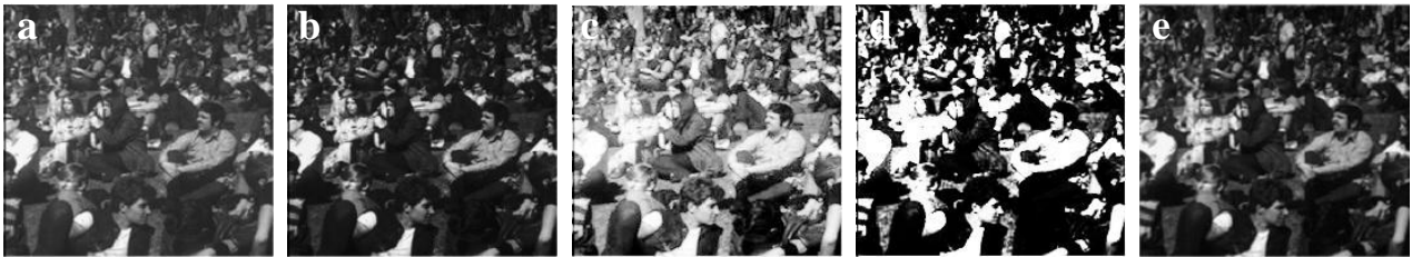
Fig 9: (a) Original crowd image; the result of the enhancement by the following methods (b) proposed method; (c) HE; (d) Contrast stretching (e) GA in [8]
