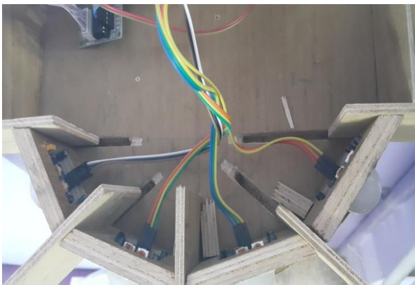
Fig. 6: Practical implementation of the sensors unit
