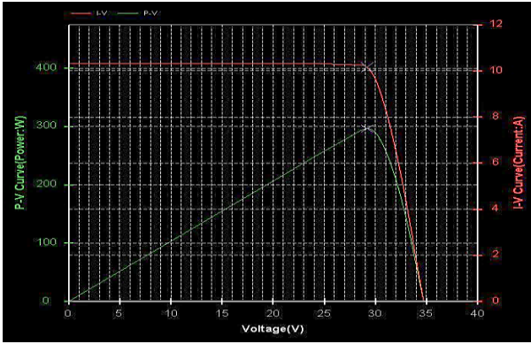
Figure (6): PV panel characteristics used in this research
