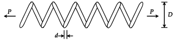
Fig. 5. Schematic view of tension/compression spring problem.
