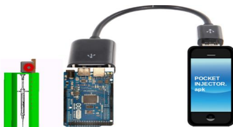
Fig 3: High Level architecture of the system
