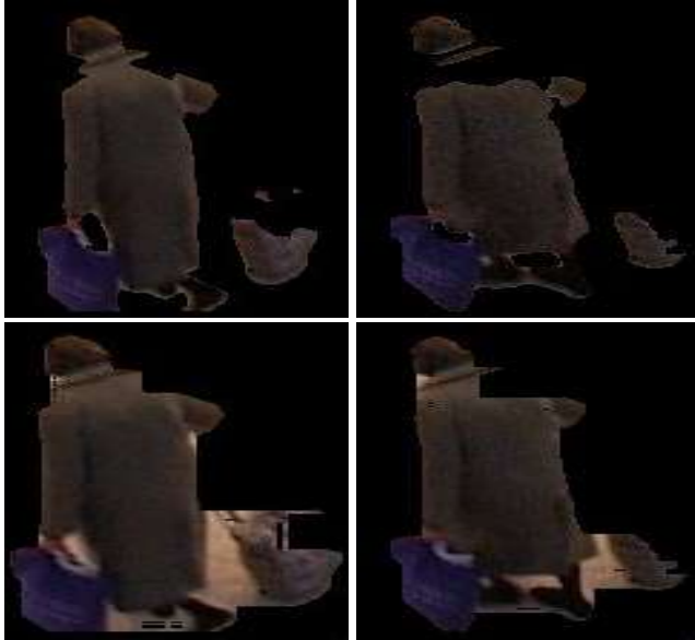
Figure 14: Frames (103 & 106) of a video Sequence of PETS 2006 data set 7, camera 3. First Row: Frames after cast shadow points are removed by the algorithm using equation (10) and (11). Second Row: Frames after spatial clustering.
