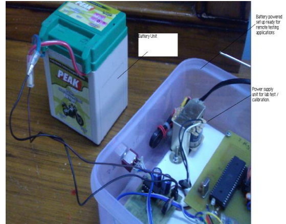
Fig.2A Battery powered unit ready for field testing / Remote Data Collection
