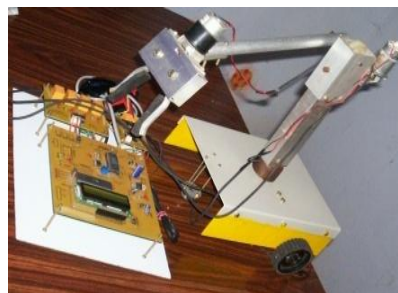
Fig 12: Fabricated sensor & Robotic arm movement interfaced with microcontroller which moves with eye blink, eyeball and EEG signals.
