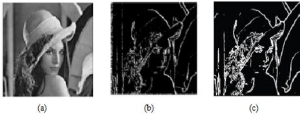
Figure. 18 (a) Original image (b) Edge detected image using rectangular Structure (c) Edge detected image using hexagonal Structure
