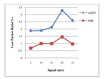
Fig 9: LPR of 60 nodes using TCP
