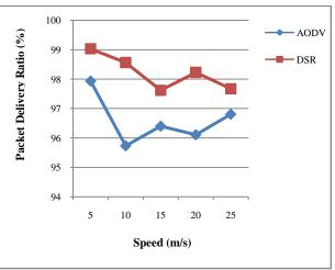
Fig 13: PDR of 90 nodes using TCP
