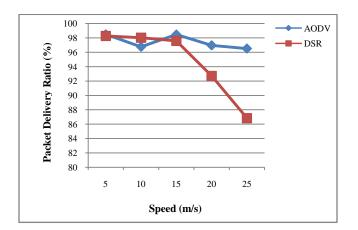
Fig 22: PDR of 120 nodes using CBR
