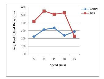
Fig 8: Avg.E-2-E delay of 60 nodes using TCP
