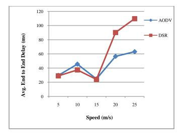
Fig 11: Avg.E-2-E delay of 60 nodes using CBR
