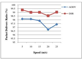
Fig 7: PDR of 60 nodes using TCP
