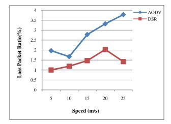
Fig 21: LPR of 120 nodes using TCP
