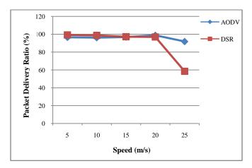
Fig 28: PDR of 150 nodes using CBR
