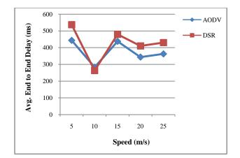
Fig 20: Avg.E-2-E delay of 120 nodes using TCP
