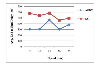
Fig 14: Avg.E-2-E delay of 90 nodes using TCP
