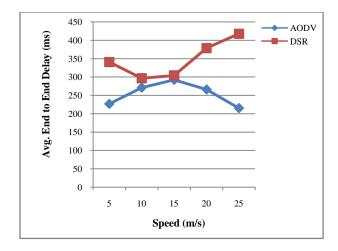
Fig 26: Avg.E-2-E delay of 150 nodes using TCP
