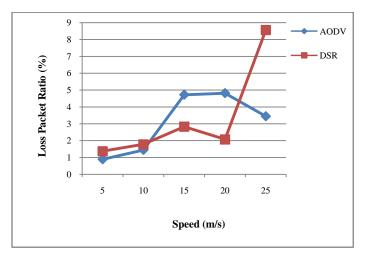
Fig 18: LPR of 90 nodes using CBR
