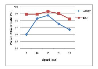
Fig 25: PDR of 150 nodes using TCP
