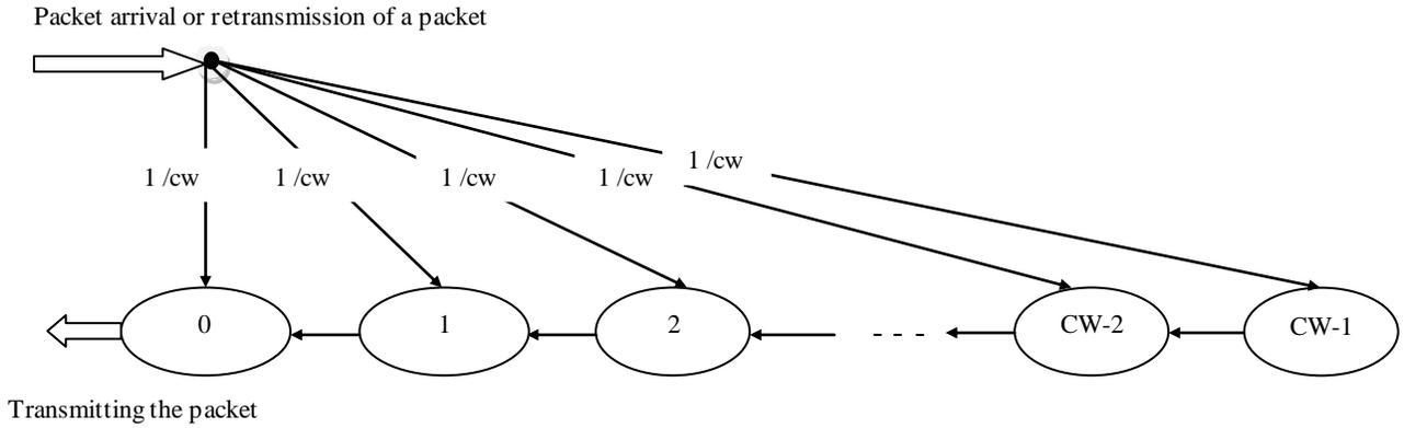
Fig 3: Markov chain model for the Backoff window size using CWA
