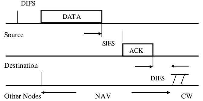
**Fig 1: Basic access mechanism in DCF**
