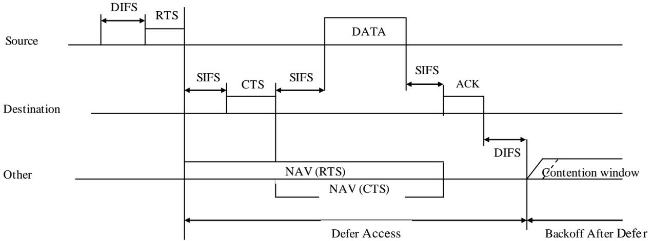
Fig 2: RTS/CTS mechanism in DCF
