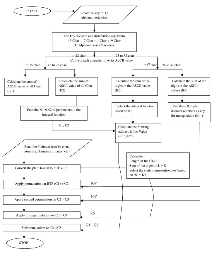
Figure 6: Flow chart for encryption process
