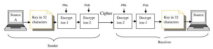
Figure 2: Secure Transmission of Key using RSA
