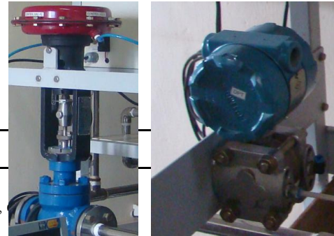
Figure 2: Images of ADAM module, Control valve, Differential Pressure Transmitter.
