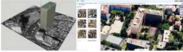
Figure 6. Left: Model of the Lotte Insurance building created in SketchUp. Right: Building model is created online in Google Earth by Google Building Marker.
